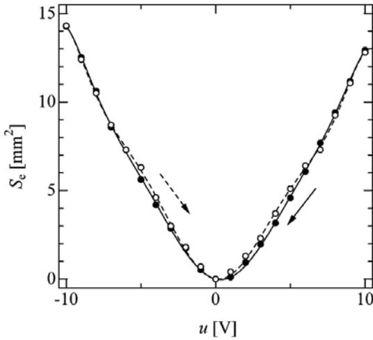
**Fig. 4** Measured results of nonlinear characteristics of the control valve
