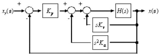
Fig. 6 Block diagram of the control system with the state feedback controller
