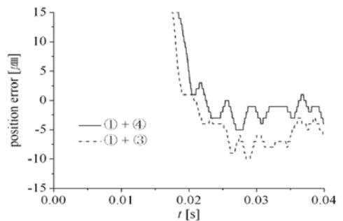
(a) Effect of the input-output characteristics of control valve on the position control accuracy
