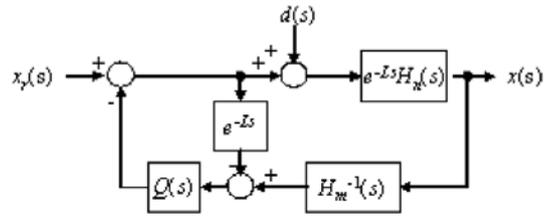
**Fig. 8** Block diagram of the control system with the disturbance observer
