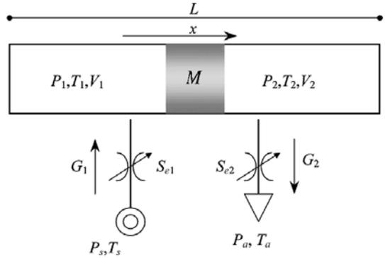
**Fig. 5** Schematic diagram of the driving apparatus
