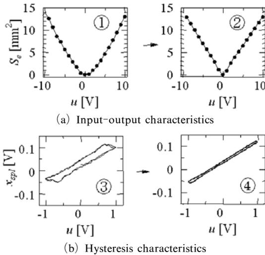
**Fig. 7** Compensated results of nonlinear characteristics of control valve using linearized input and dither signal
