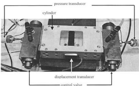
Fig. 1 Configuration of the pneumatic cylinder driving apparatus
